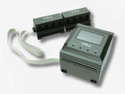
The DC-Monitor product is mainly used in DC power transmission and distribution, such as combiner boxes and DC cabinets. Its main function is the real-time monitoring of the generation current, voltage, temperature of the combiner box, lightning arrester status, DC circuit breaker status, and DC Arc Fault Status of each photovoltaic string in the combiner box. It communicates with the host computer through RS485.
